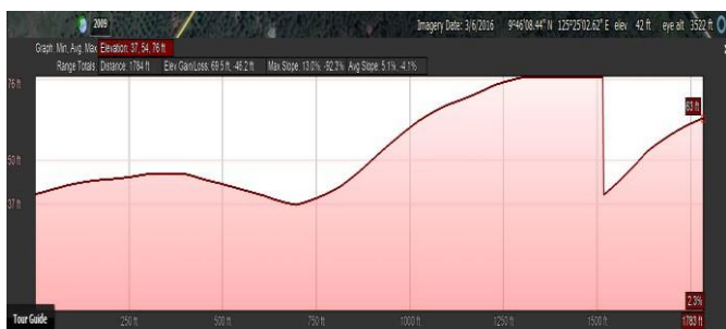
Fig. 6. Elevation Profile between the AP (Bgy. Hall) to STA1 (Principal's Office)
