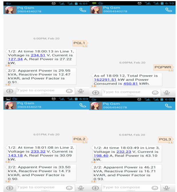
Fig. 9. Graphical User Interface for Remote Accessing via Internet or SMS
