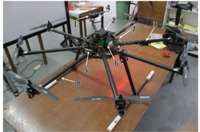
Legend: [1]GPS Antenna [2]Raspberry + Navio+ [3]RC Receiver [4]Telemetry Radio Receiver [5]UBEC [6]Battery Pack [7]Power Module [8]Landing Gear V2
