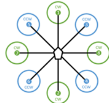
Motor Orientation: Pitch – Motors 5, 7 and 6 vs Motor 3, 8 and 4 Roll – Motors 5, 1 and 3 vs Motor 6, 2 and 4 Yaw – Clockwise (CW) vs Counter-clockwise (CCW)
